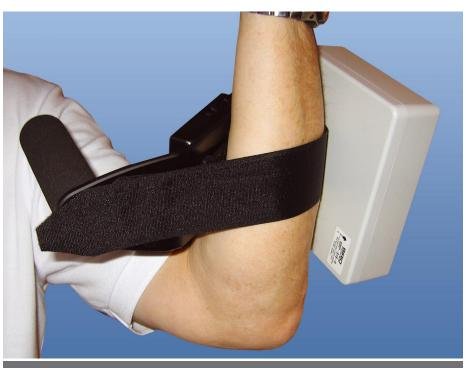
The GSM196 when used with the SA918 allows the officer to scan a specific direction with rejection of signals in all but the direction the antenna is pointing.
