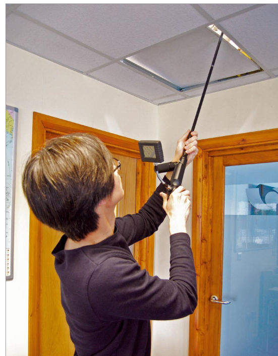
Rigidizer quickly converts videoscope into pole camera
